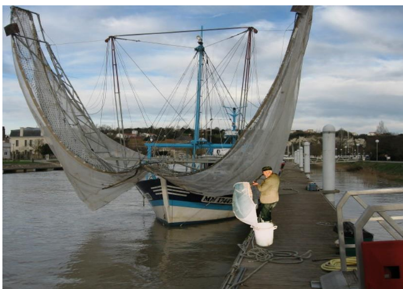
Figure 4 - A comparison between the trawl used in the French estuaries and a dip net used in the Severn (UK dip net in the foreground)
